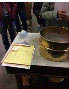
Sieves are used to finish the seed, removing as much inert material as possible.
